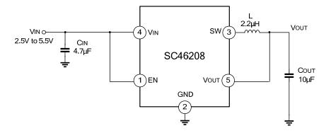
Fig.2: Output voltage fixed regulator
